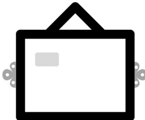
Mirror plates attached to the midpoint of frame Label attached to the back of work
